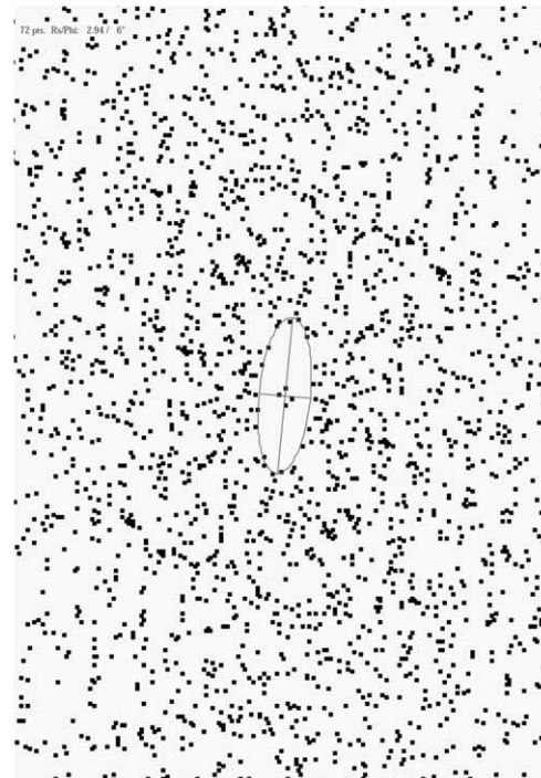
Fig. 11. Fry analyses from sections of two hand specimens of the Cesson Conglomerate, using scans of two serial sections of each, 10 \times 15 to 10 \times 20 \text{ cm}^2 in size: (a, b) cut parallel to XZ; (c, d) cut parallel to YZ. Best-fit ellipses are outlined on each figure, and the R_s results shown for each, also in Table 3d.
